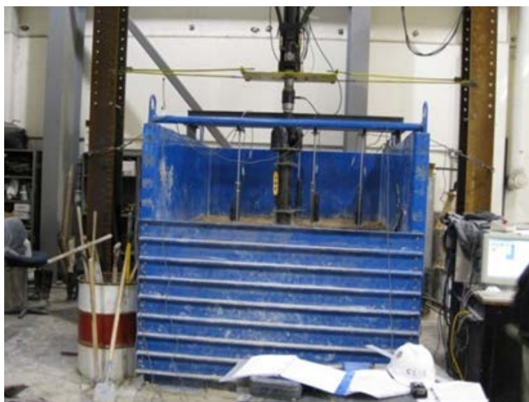
Figure 1. Large-scale geotechnical box for cyclic plate loading tests
