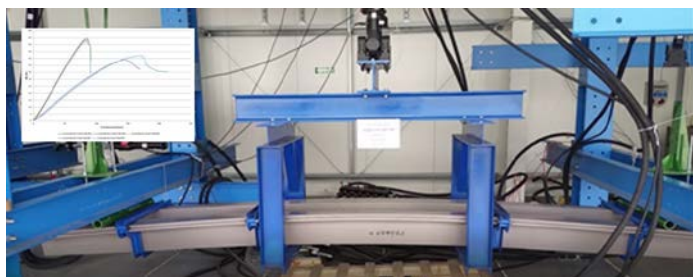
The static and fatigue tests included 4-point bending of the profile using a specially designed testing unit
