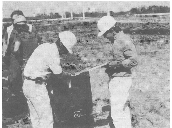
Tommy C. Bradford (left) and Daniel A. Schauer (right), CQA personnel of GeoServices, preparing a polyethylene geomembrane sample for conformance testing.
