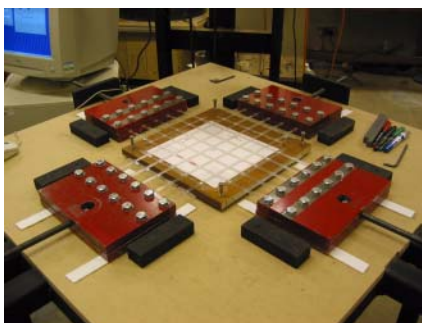
Biaxial sustained loading (creep) test apparatus.
