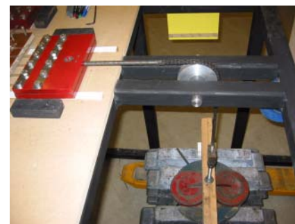
Biaxial sustained loading (creep) test apparatus.
