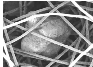
Figure 4. Impregnated geotextile under 2 kPa (left) and 1,000 kPa (right). Figure 5. Large particle in a geotextile void.
