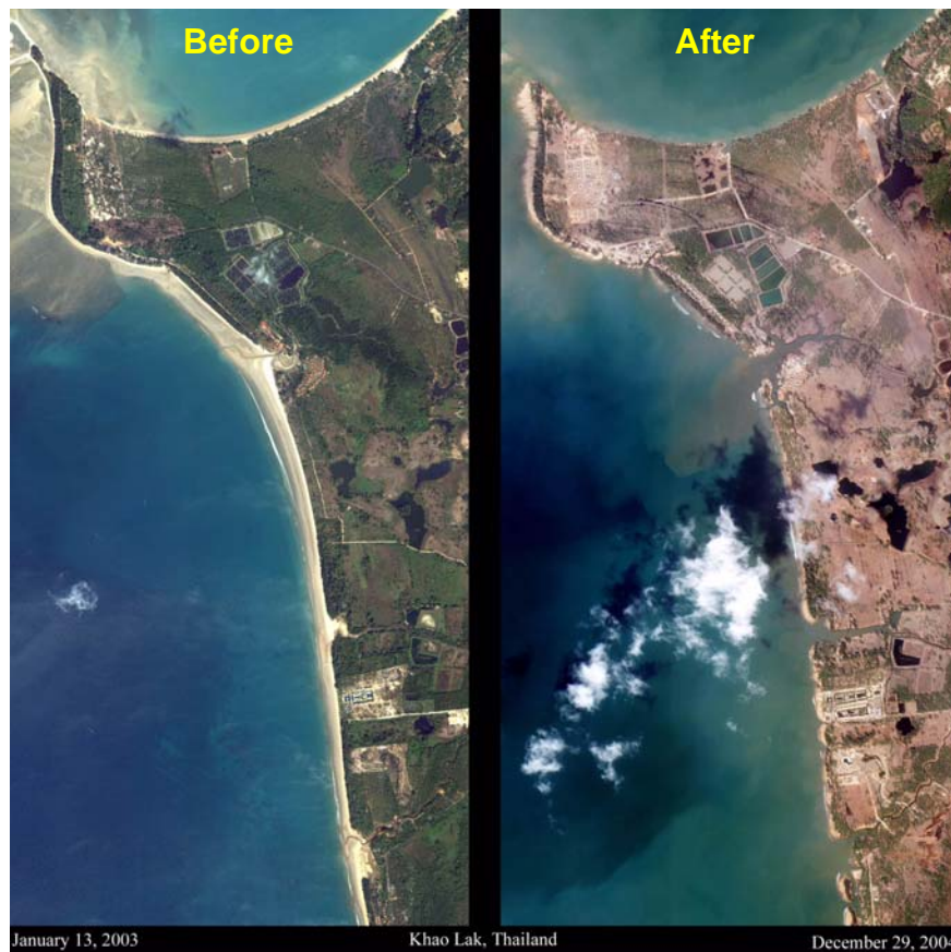
Figure 2. Coastal erosion due to tsunami in Khao Lak, Phanga, Thailand.
