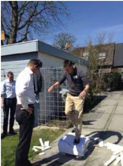
Photo's 4 Two model piled embankments performed well.
