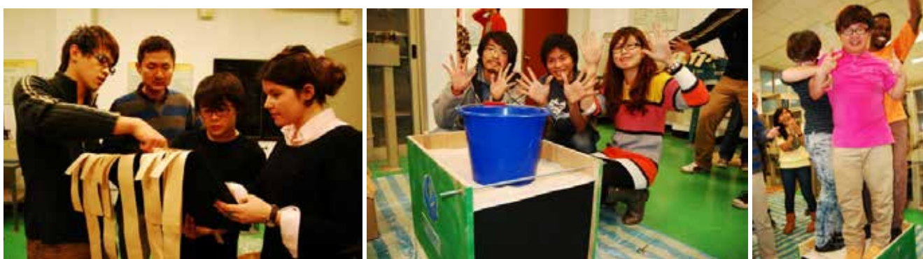
Figure 5. Small-scale paper MSE wall competition: (left to right) discuss on students' design; place 25kg surcharge; success after placing large loading (three people stand on the top of the paper MSE wall).
